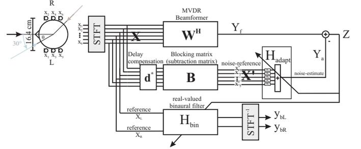
Abbildung 1: GSC beamformer and binaural post-filter
